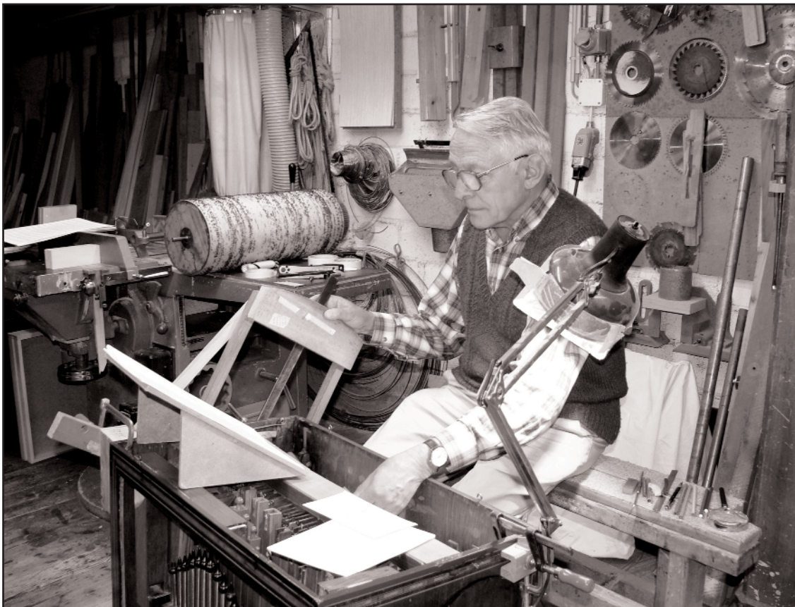
Figure 8. Martin Zumbach at work pinning a new barrel for a Violinopan.
